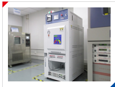
Highly accelerated stress test
